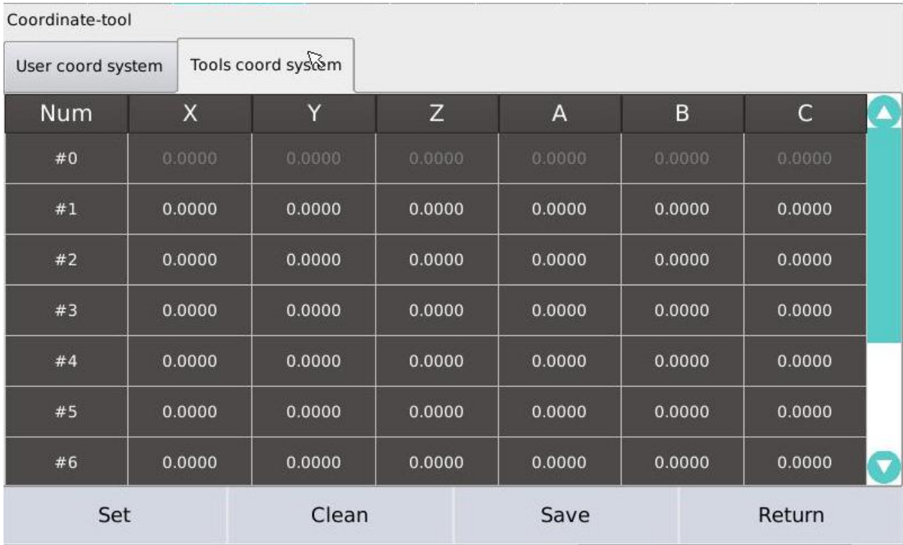
FIG. 5-3-1-3 Tool coordinate system
