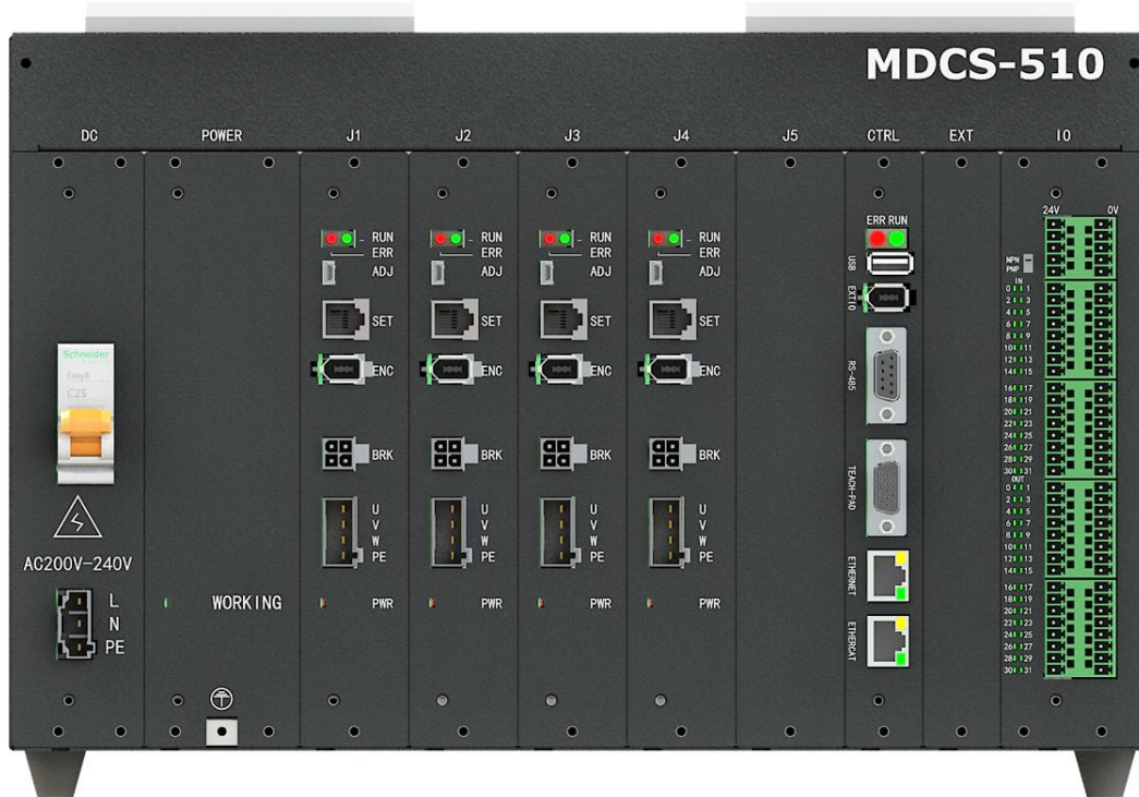
FIG. 2-2 terminal panel layout
